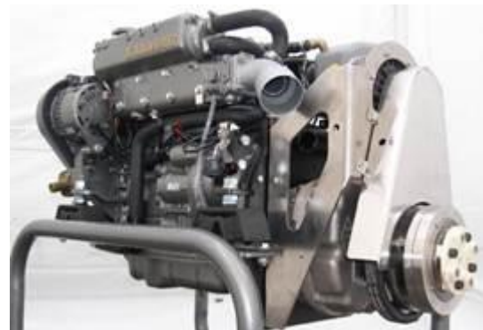
Figure 11 Yanmar hybrid engine developed by Hybrid Marine, UK
